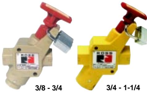
Manual L-O-X<sup>®</sup> valve shown padlocked in closed position. The valve can only be locked in the closed position. The position of the red handle indicates full flow pressurizing or exhausting capability.
