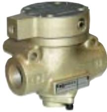
The EEZ-ON® valve is designed to allow a gradual buildup of downstream air pressure before opening to full air flow. This gradual pressure buildup allows cylinders or other work elements to move slowly and more safely into their normal working positions before full line pressure is applied. An adjustable restriction within the EEZ-ON® valve determines the rate of downstream pressure buildup, and consequently the time delay for the full opening of the EEZ-ON® valve.
