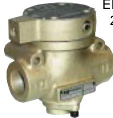
EEZ-ON® valves are available as either 2/2 (2-port, 2-position) or 3/2 (3-port, 2-position) valves. Either type can be used in conjunction with a L-O-X® valve to supply a lockout and exhaust feature in addition to the gradual buildup of supply pressure.
